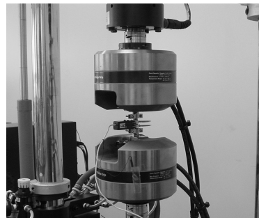
Fig. 2 Photograph of low cycle fatigue test with anti-buckling device
