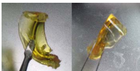
Fig. 3. Photographs of free standing SPE5 sample after vacuum dry at 80°C for 72 hours.
