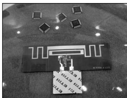
Fig. 7. (c) ETRI's sensor tag and 3.0 V-class film battery.
