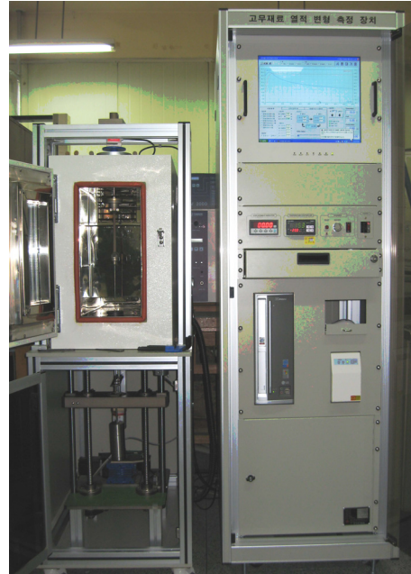
Figure 2. A schematic diagram and the test machine for measuring thermal stress of rubbery materials upon heating: ①chamber, ②clamps, ③load cell, ④rod, ⑤LVDT, ⑥screw, ⑦crosshead and ⑧motor.
