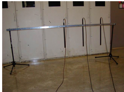
Fig. 2 Test setup showing microphones and the rack mount (Zhu and Popovics, 2005)
