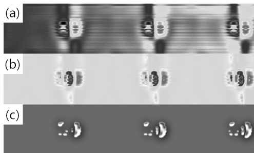
Fig. 18 In the case of no crack; (a) Normal, (b) \partial V/\partial x , (c) Image processing
