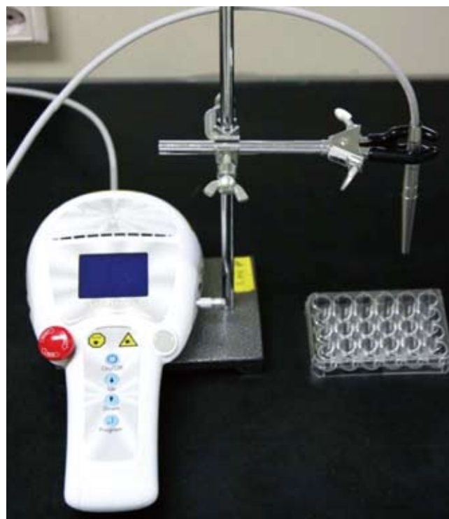
Figure 1. A gallium-aluminum-arsenate semiconductor diode laser with an 810-nm wavelength was prepared and the fiber tip was perpendicularly positioned at a 10-cm distance from the cell monolayer.
