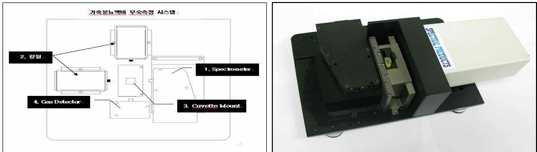
Fig. 5. Scheme and picture of measuring system for fermentation degree of liquid swine manure.
