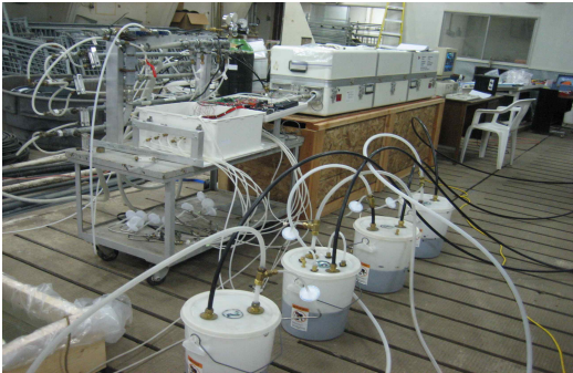
Fig. 3. Pails storing liquid swine manure and TGA systems.
