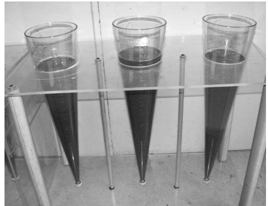
Fig. 3. Difference of sludge accumulation in pig slurry by application type of media.
