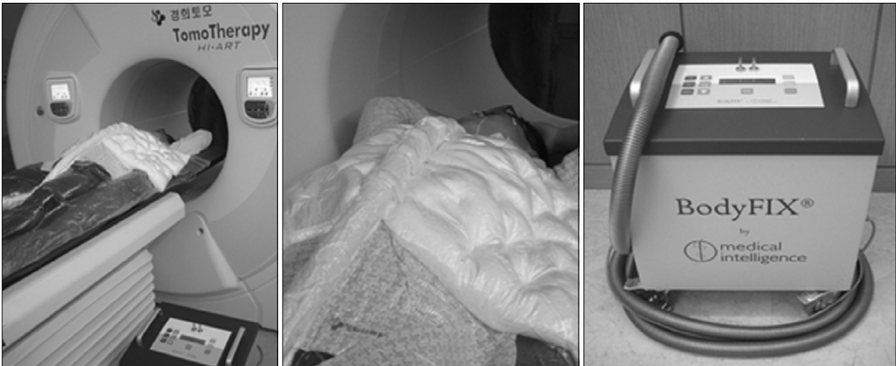
Fig. 2. The Body-fix immobilization system. The air among the clear plastic sheet, patient, and the whole body vac lock was evacuated covering the patient's lower body up to the abdomen with the clear plastic sheet.
