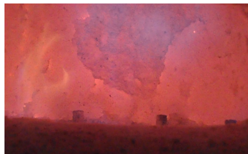
Figure 5: A flame photograph of MILD combustion mode at \Phi=0.64
