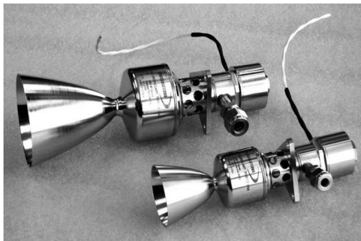
Fig. 7 FM model thrusters (100, 250 N class)
