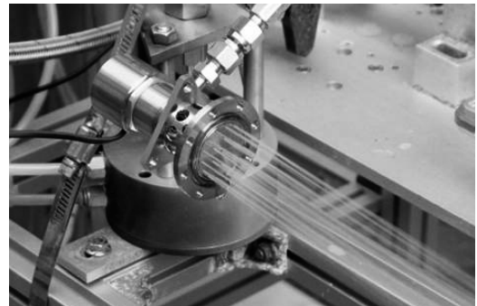
Fig. 8 Injector water flow test at FM model
