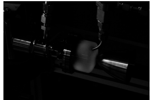
Fig. 9 Reaction test apparatus with FM thruster
