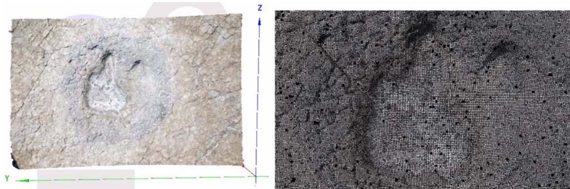
Fig. 4. 3D images included point cloud after superimposed stereoscopic image pair of Fig. 3.
