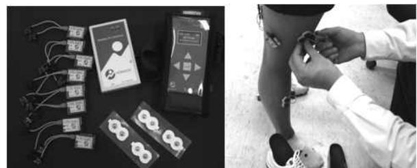
Figure 3. TeleMyo DTS telemetry system(Noraxon)
