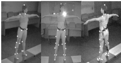
Figure 1. Marker attachment point of body joints and segments
