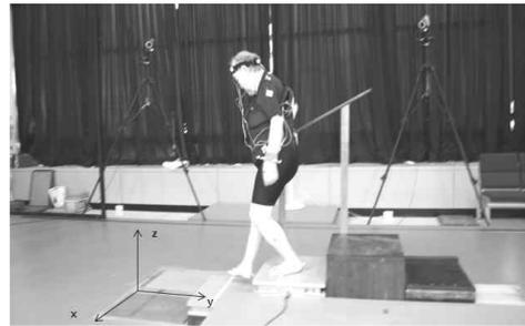
Figure 3. Real trial of down staircase walking & Global reference frame setup
