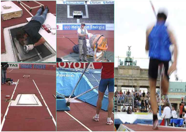
Figure 1. Set up of dynamometric planting box during the 2005 Helsinki IAAF World Championships in Athletics.
