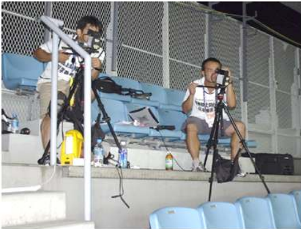
Figure 3. Example of Setting the 5 Lavegs in seat during the 2007 Osaka IAAF World Championships in Athletics.
