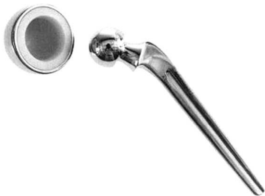
Fig. 3. The bipolar shoulder implant allows motion between a distal extremity and a proximal part through two moving interfaces. The ball of the intramedullary stemmed humeral component articulates with a polyethylene bearing within the glenoid cup component. The glenoid component has the advantage of not being fixed to bone. (Swanson AB, de Groot Swanson G, Sattel AB, Cendo RD, Hynes D, Jar-Ning W: Bipolar implant shoulder arthroplasty. Long-term results. Clin Orthop Relat Res, 249: 227-247, 1989.) 35)
