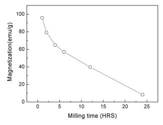
**Fig. 2.** Variation of magnetization for  $Fe_{50}Cr_{50}$  powders with increasing milling times.
