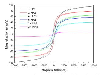
**Fig. 1.** M-H curves for  $Fe_{50}Cr_{50}$  powders with increasing milling times.
