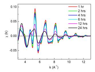
**Fig. 3.** EXAFS spectra of  $Fe_{50}Cr_{50}$  alloys with indicated milling times.
