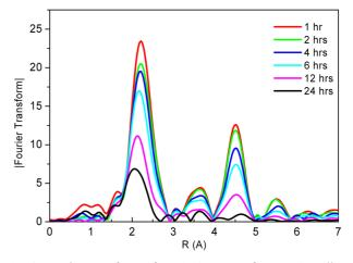
**Fig. 4.** Fourier transform of EXAFS spectra for  $Fe_{50}Cr_{50}$  alloys measured at Fe K-edge with indicated milling times.
