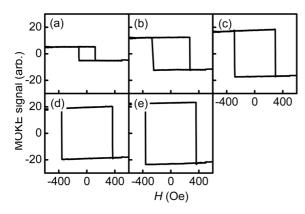
**Fig. 1.** Out-of-plane magnetic hysteresis loops of the films with different repetition numbers *n* of the CoFe/Pt layers, i.e. n = (a) 1, (b) 2, (c) 3, (d) 4, and (e) 5, respectively. The sweeping rate of the magnetic field is 66 Oe/sec within the range of  $\pm 2,400$  Oe. The coercive field of each film was measured to be (a) 113 Oe, (b) 272 Oe, (c) 295 Oe, (d) 360 Oe, and (e) 363 Oe, respectively.
