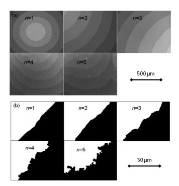
**Fig. 2.** (a) Typical magnetic domain expansion from nucleation sites, which are sometimes at the edge (or middle) of the film, with low magnification ( $\times 25$ ). The gray contrasts correspond to the domain images taken at different times after applying the magnetic field. (b) Typical magnetic domain images with high magnification ( $\times 1,000$ ) after image processing, which comprises background subtraction and black-and-white conversion.
