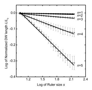
**Fig. 3.** Log-log plots of the domain wall length with respect to the ruler size for each film. The symbols with error bars indicate the statistics from several tens of images for each film. The lines show the best linear fits.
