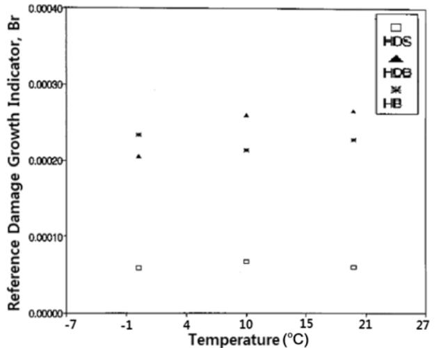
Fig. 6. Reference damage growth indicator ( $B_r$ ) versus temperature.
