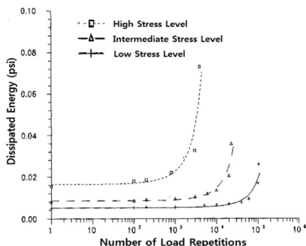
Fig. 2. Dissipated energy versus number of load repetitions in controlled-stress tests.
