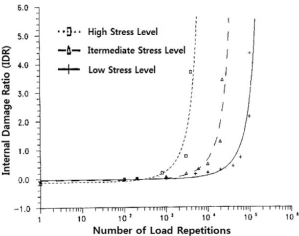
Fig. 3. Internal damage ratio versus number of load applications with HDS mixture at 0°C.
