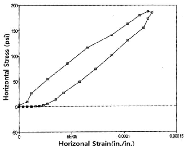
Fig. 1. Typical stress-strain hysteresis loop at 0°C
