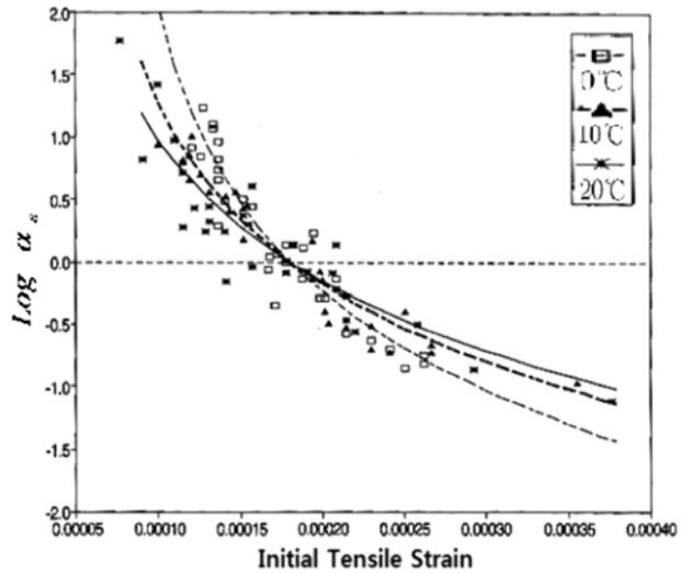
Fig. 5. Log versus initial tensile strain with introduction of threshold tensile strain at three temperatures(0, 10, and 20°C).
