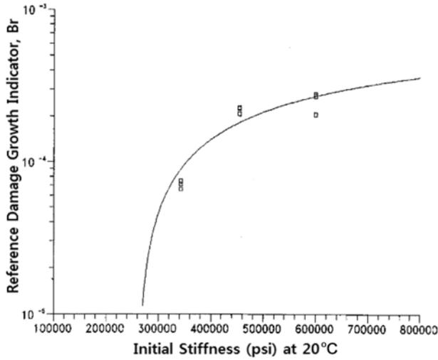
Fig. 7. Initial mixture stiffness ( $S_i$ ) versus reference damage growth indicator ( $B_r$ )
