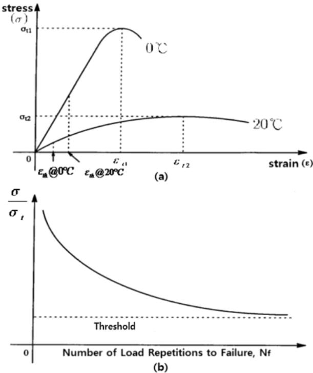
Fig. 4. General concept of threshold tensile strain(Kim, N., 1994).
