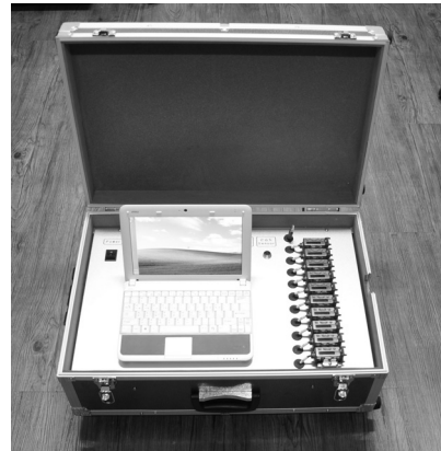
Fig. 4. Main controller of rock fall monitoring system
