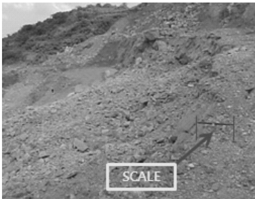
Fig. 17. Fine fragmentation & throw at high stiffness ratio (linear scale 0.5 m).
