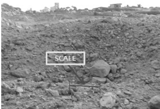
Fig. 12. Good fragmentation within the well displaced muck pile (linear scale 0.5 m).
