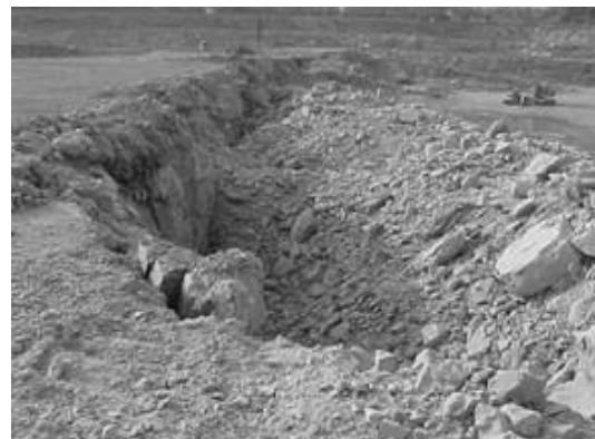
Fig. 14. Good throw and uniform fragmentation (diagonal firing).
