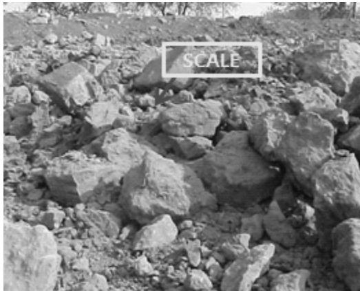
Fig. 1. Occurrence of large over sizes within a blasted limestone muck pile (square scales 0.5 m x 0.5 m)
