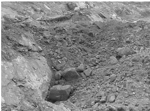
Fig. 11. Good throw & drop in the limestone quarry (straight V- type firing).
