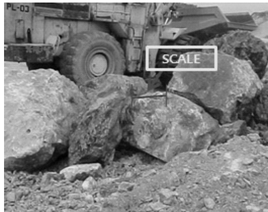
Fig. 4. Separated over sizes for secondary breakage (linear scale 0.5 m).
