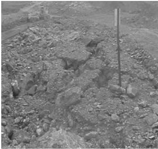
Fig. 6. Network of back breaks.
