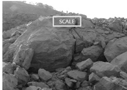
Fig. 13. Poor fragmentation results in a limestone quarry (row- to- row firing square scale 0.5 m x 0.5 m).
