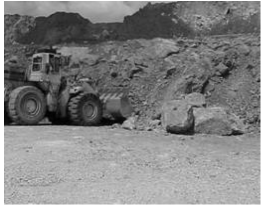
Fig. 3. Front-end-loader operation vis-à-vis presence of over sizes.
