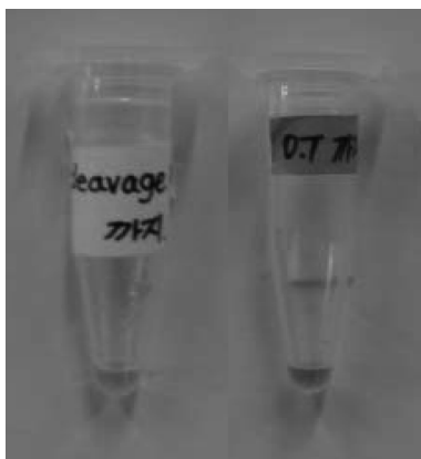
Fig. 2. Representative characterizations of the resins using the Kaiser test: characterization indicative of a complete coupling reaction (left) and an incompletely coupled resin (right).
