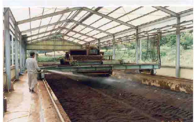
Fig. 1. Production of antifungal compost by spraying of B. licheniformis KJ-9.
