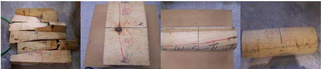
Fig. 3. Failure types for the pine skin timber.(specimen1, 2, 3, 4)
