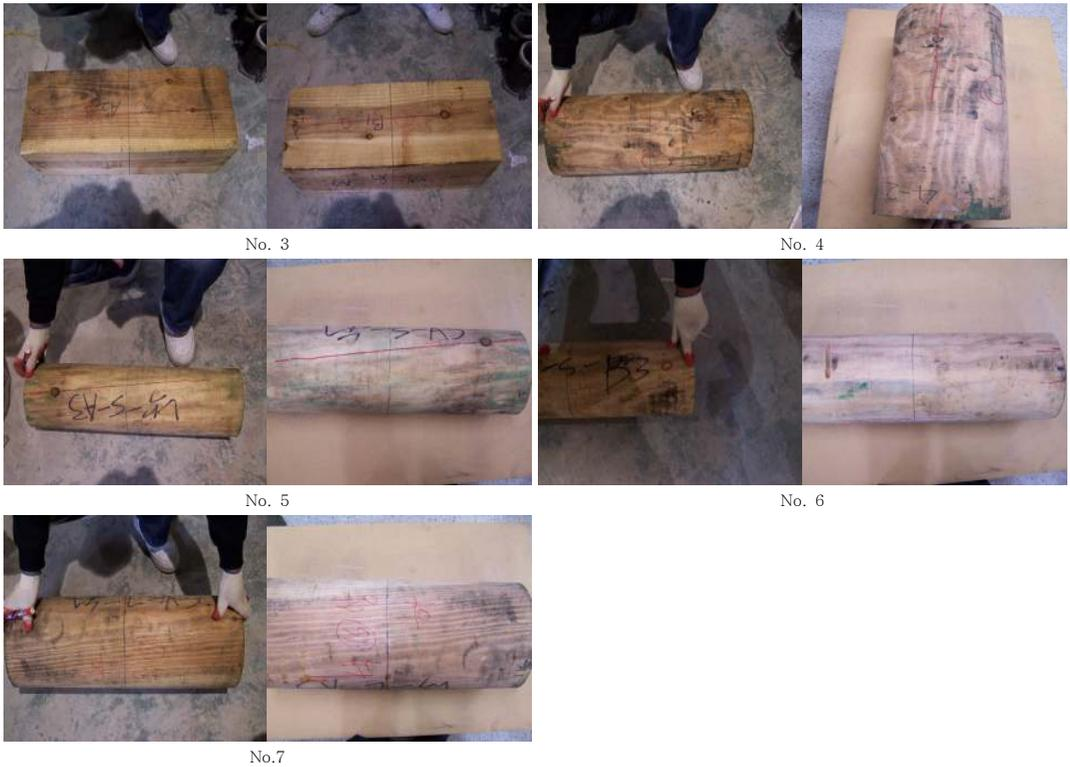
Fig. 6. Failure features for the larch skin timber.
