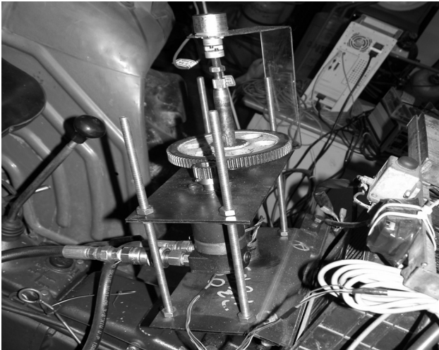
Fig. 2 Hydraulic system for driving the column axle.
