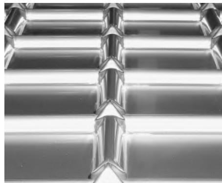
Fig. 1. Typical membrane panel.
