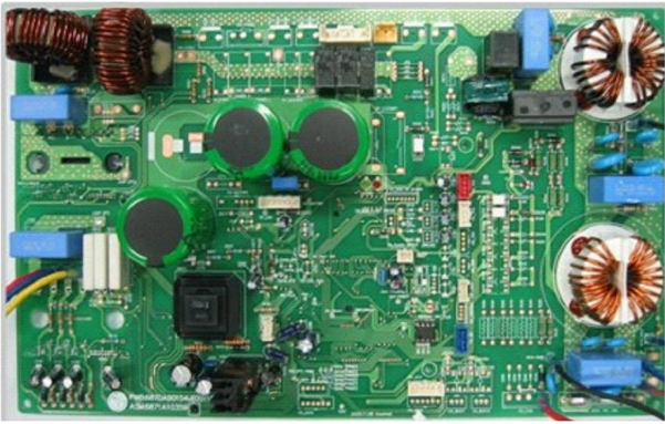
Fig. 15. Prototype of DC inverter control system.
