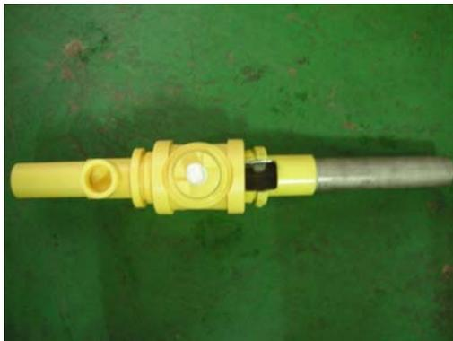
Fig. 8. Unified ball valve and polyethylene-steel pipe with partial dissection.
