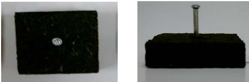
Fig 5. Specimen of nail withdrawal test
