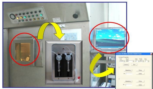
Fig. 4. Radiopharmaceuticals automated divider was placed inside hot cell and cable chords were used in the equipment, and then it was connected to PC outside hot cell to make it possible to control the 18 F-FDG automated divider.
