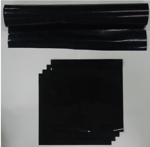
Fig. 4 Manufactured EM wave absorber.
