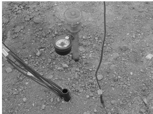
Fig. 4 Measurement of soil potential energy.
