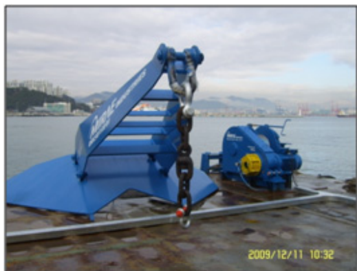
Fig. 5 Embedment drag anchor & positioning winch
