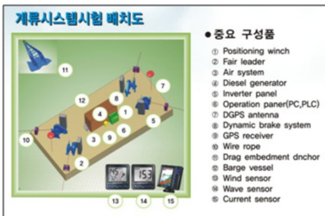
Fig. 2 Arrangement of the ship-to-ship SMS equipment on board a Barge
