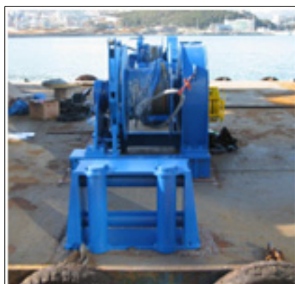
Fig. 6 A fairleader & positioning winch
