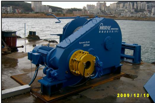
Fig. 11 Developed positioning winch for MH
