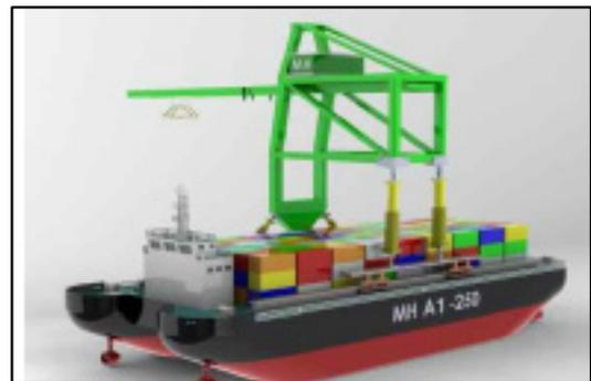
Fig. 5 ZMSC(Zero Moment Stabilized Crane)
