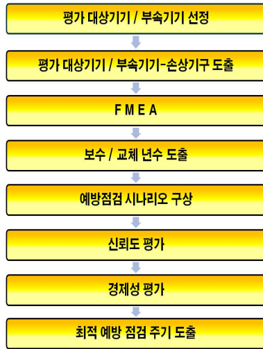
Fig. 6 Overall flow chart of process to optimize preventative maintenance cycle of pumped-storage power equipments.
