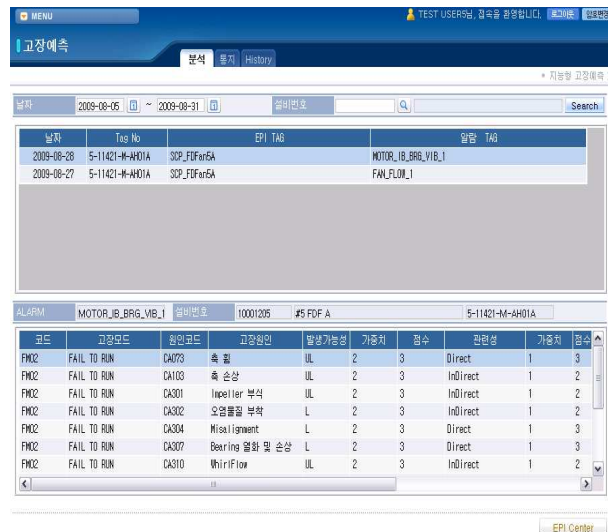
Fig. 8 Screen for failure monitoring and prediction
