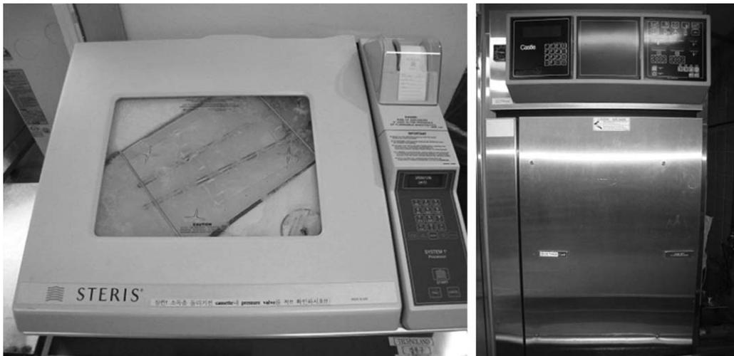
Fig. 5. (A) Steris System 1® (Liquid chemical sterilization) (B) EO gas 소독기
