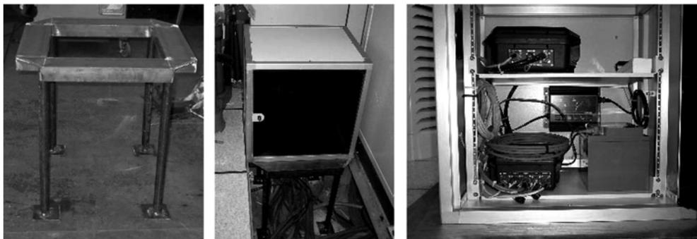
Fig. 4. Support frame and interior of the rack for housing a recorder system.
