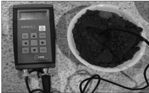
Fig. 3. TDR sensor to measure water content ratio.
