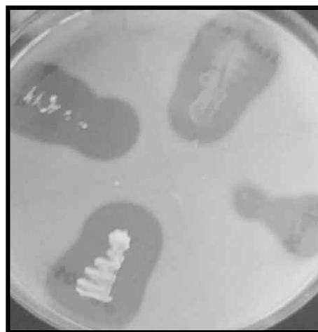
Fig. 1. Screening of lipase production by selected bacterial isolates using tributyrin agar plate assay method.
