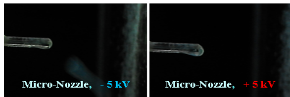
(a) Drop formation mode [ V_{DC}=\pm 3\sim 5 kV]
