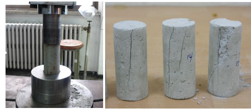
Fig. 1. Measurement of uniaxial compressive strengths.
