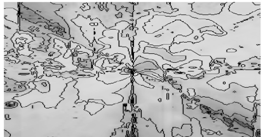
Fig. 9 Field computed by second order rays for horizontal polarization ( cl=50 m, dv=5 m, sl=1 Km).
