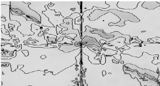
Fig. 7 Field computed by first order rays for horizontal polarization ( cl=50 m, dv=5 m, sl=1 Km).
