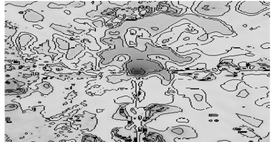
Fig. 8 Field computed by second order rays for vertical polarization ( cl=50 m, dv=5 m, sl=1 Km).
