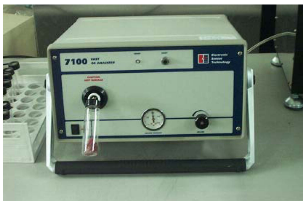
Fig. 1. The SAW based an electronic nose system for detecting Salmonella odor from beef sample.
