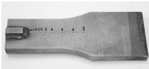
Fig. 4 Configuration of specimen and the measurement points
