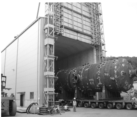
Fig. 9 Photo of large scale furnace for PWHT
