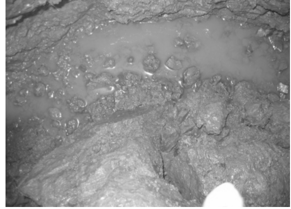
Fig. 3. Percolated water in the slide zone
